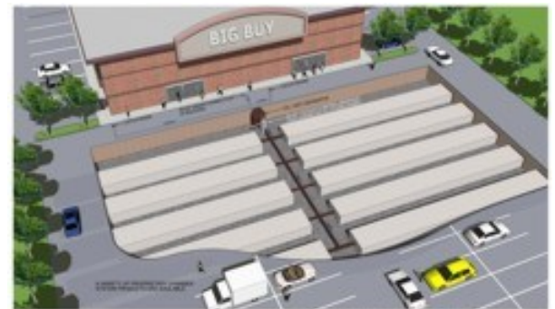
Parking Lot Infiltration Chamber (Image source: Schollen and Company)
